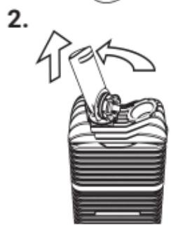
Put the edge of the Mouthpiece into the notch of the Rotary Cap and turn it counterclockwise to open and pull out. Pull off the Seal Ring from the Rotary Cap using the recess.
