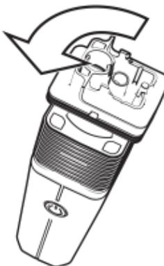
Unscrew the Cooling Unit Base from the Vaporizer by turning it 90° counterclockwise.
