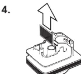
Pull out the Screen inside the Cooling Unit.
