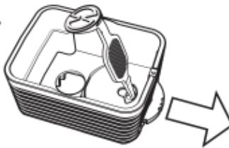
Use the Filling Chamber Tool to press the Setting Wheel out of the Cooling Unit.
