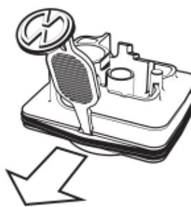
Lever out the large Base Seal Ring with Filling Chamber Tool at the recess in the groove.
