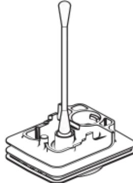
Carefully press out the Screen from above using a cotton swab.
