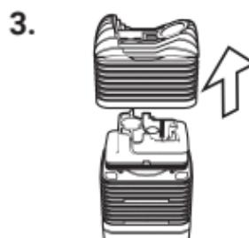
Pull the Cooling Unit Cap off the Vaporizer.
