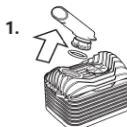
Pull the Mouthpiece out of the Cooling Unit Cap while slightly tilting it back and forth. Pull off the Mouthpiece Seal Ring using the recess.
