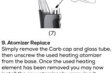
element has been removed you may now install the new atomizer by screwing it directly into the device. Then re-install the glass tube and carb cap. You may need to press the atomizer a little bit when installing the new coil, because the atomizer use a spring thread.
