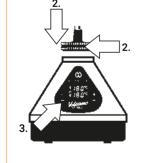
2. Screw on Filling Chamber. 3. Switch heat on.
